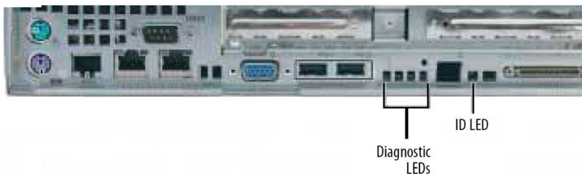
Figure 3-24. Rear I/O Panel Controls and Indicators
